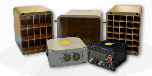
CMDS is used to provide self-protection for the host platform against radar- and infrared-guided weapon systems by autonomously or manually deploying appropriate countermeasures. It operates in coordination with other onboard selfprotection systems such as the Radar Warning Receiver (RWR) and the Missile Warning System (MWS), based either on pilot commands or autonomous threat detection.
